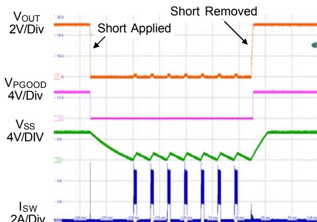
Figure 3. Short Circuit Protection and Recovery
