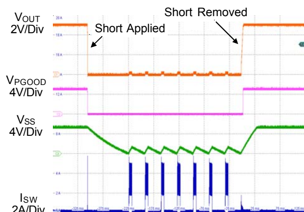
Figure 3. Short Circuit Protection and Recovery
