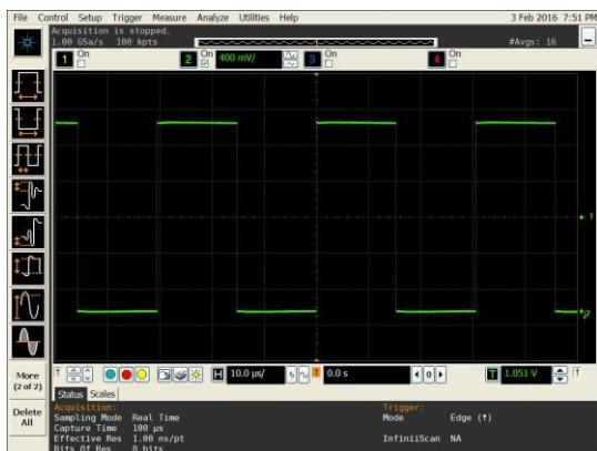
Figure 3. LVC MOS Output Swing ( V_{DD} = 1.8\text{ V} )
