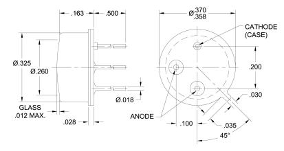
All surfaces are gold plated. Dimensions are nominal values in inches unless otherwise specified. Two Anode pins *must be* externally connected together.
