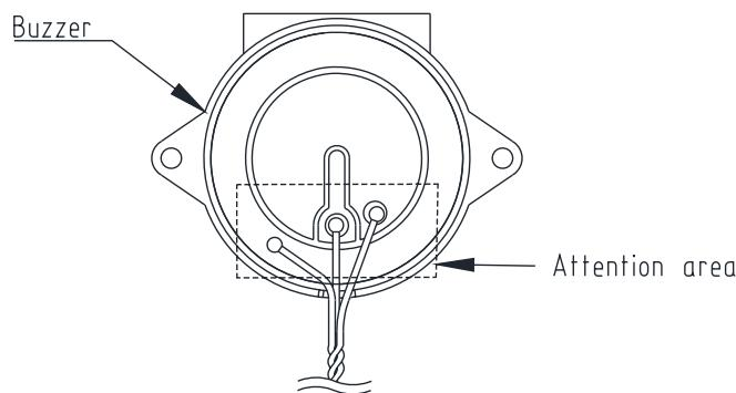
If buzzer's piezo side close to any potentially conductive surface, it is recommended that the product body surface (not piezo side) should add insulating tape to prevent short circuit conditions.
