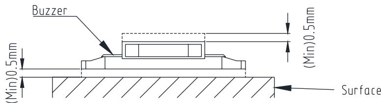
It's recommended reserve at least 0.5mm between the product and the surface. And the surface must not have any protrusions.
