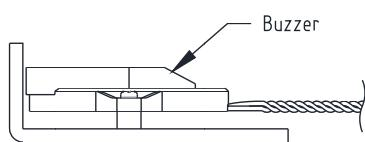
The buzzer should be as close as possible to the front case or the SPL will decrease. And we suggest the design of the sound hole should be simple.
