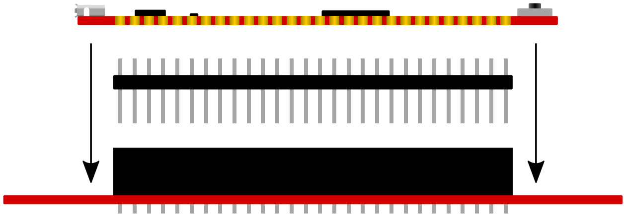
Figure 4-4. Connecting to Curiosity Nano Base for Click boards™
