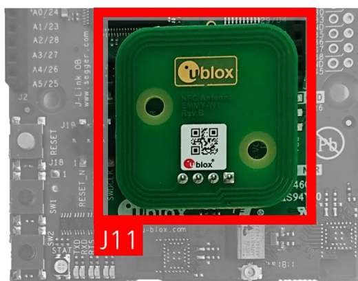
Figure 3: Left: EVB ANNA-B112U including NFC antenna; Right: EVB ANNA-B112U including NFC antenna, turned 180 degrees. Both options are valid.
