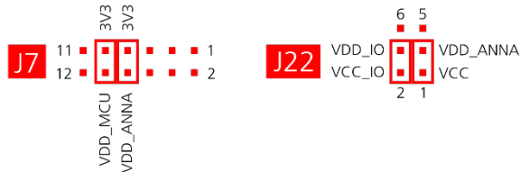
Figure 8: Jumper positions for default power configuration
