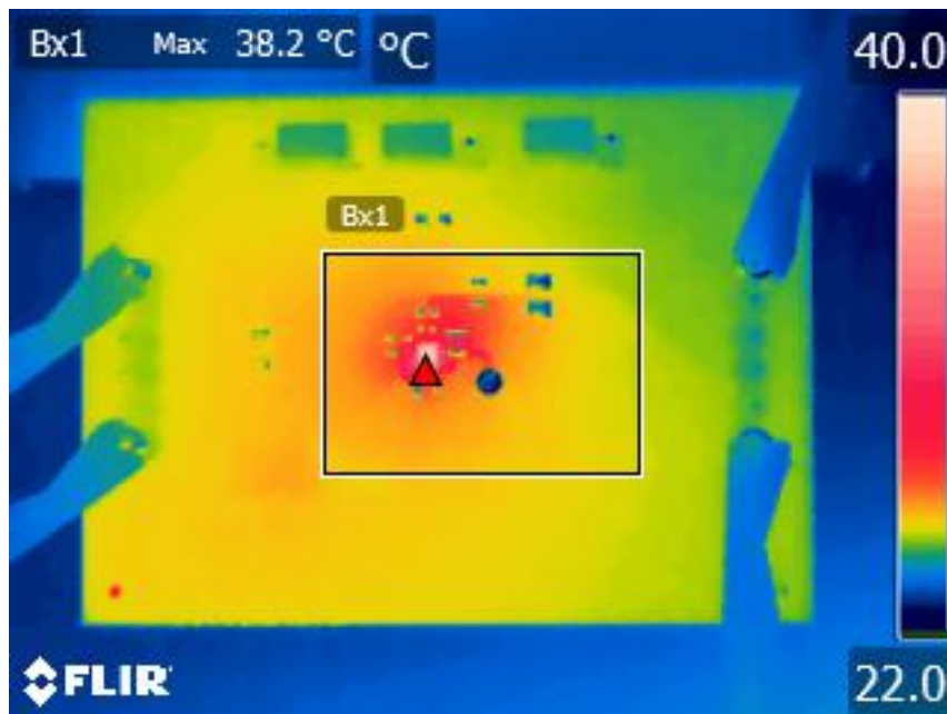
Figure 2. TPS62840 Thermal Performance ( V_{IN} = 3.6\text{ V} , V_{OUT} = 1.8\text{ V} , I_{OUT} = 750\text{ mA} )
