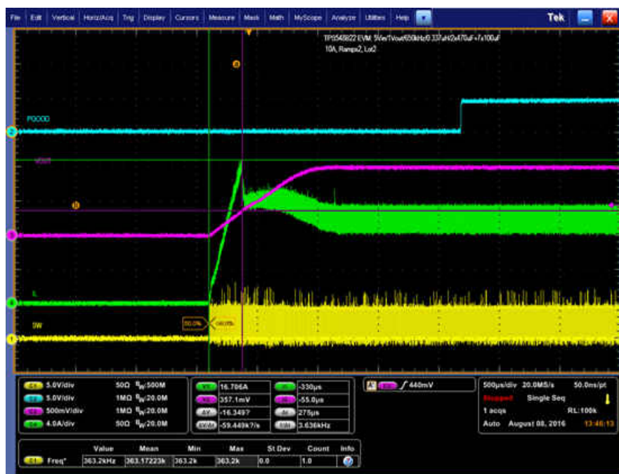
Figure 11-13. 0.5-V Pre-bias start up from Control, 1-V Output at 12 V IN , 10-A Output
