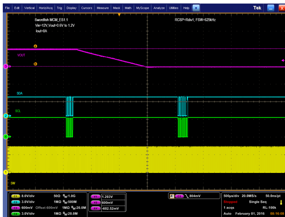
Figure 11-5. PMBus V OUT Step-Down = 1.2 V to 0.6 V at 0 A
