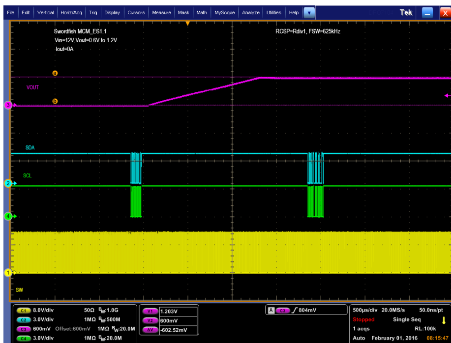
Figure 11-4. PMBus V_{OUT} Step-Up = 0.6 V to 1.2 V at 0 A
