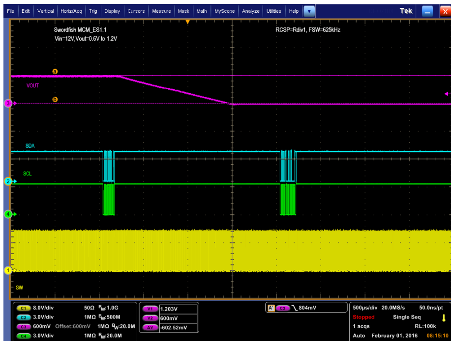
Figure 11-7. PMBus V_{OUT} Step-Down = 1.2 V to 0.6 V at 25 A
