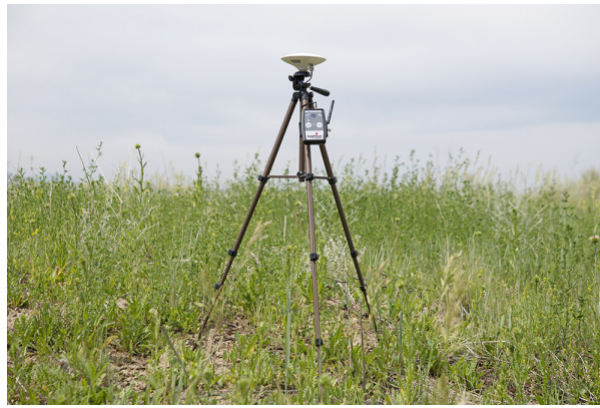
Temporary RTK Express Base setup
