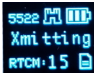
RTK Express in Fixed Transmit Mode
