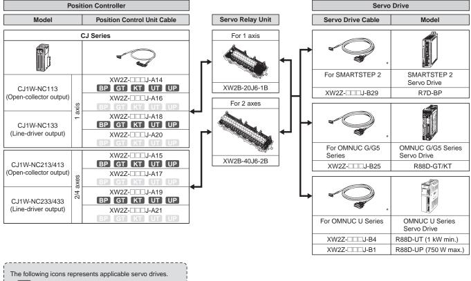
The following icons represents applicable servo drives. BP : SMARTSTEP2 GT : OMNUC G Series KT : OMNUC G5 Series UT : OMNUC U Series (1 kW min.) UP : OMNUC U Series (750 W max.)
