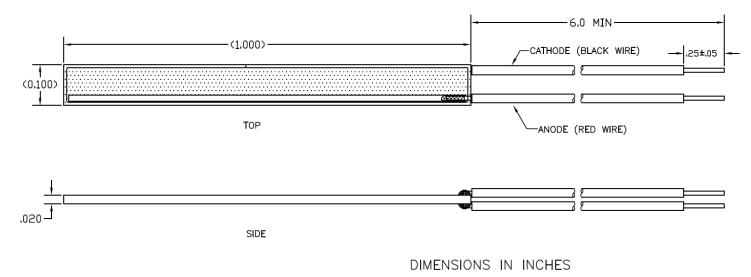
> Soldering Conditions: 260°C 1/16 inch away from case for 3 seconds max.
