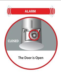
Because the magnet ball contact will not weld, when the door is opened the contact will close and the **SYSTEM WILL ALARM.**
