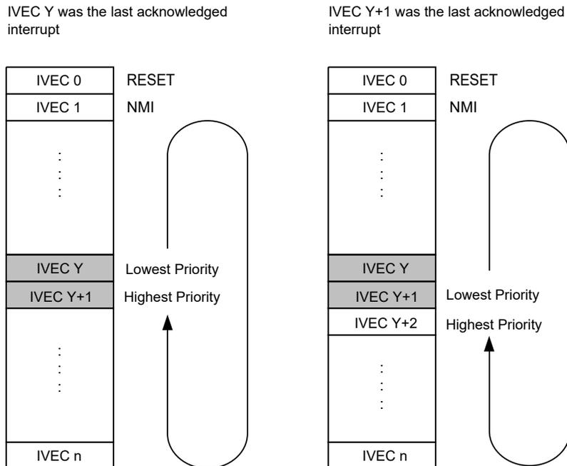
The round robin scheduling for LVL0 interrupt requests is enabled by writing a '1' to the Round Robin Priority Enable (LVL0RR) bit in the Control A (CPUINT.CTRLA) register.
