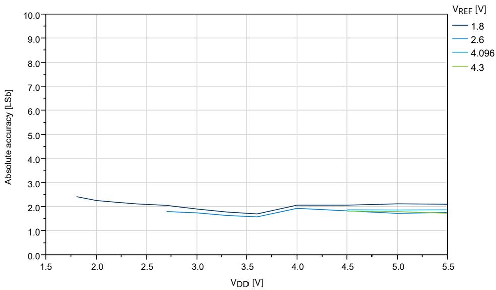
**Figure 33-55. Absolute Accuracy vs.  $V_{REF}$  ( $V_{DD} = 5.0V$ ,  $f_{ADC} = 115$  kps, REFSEL = External Reference)**
