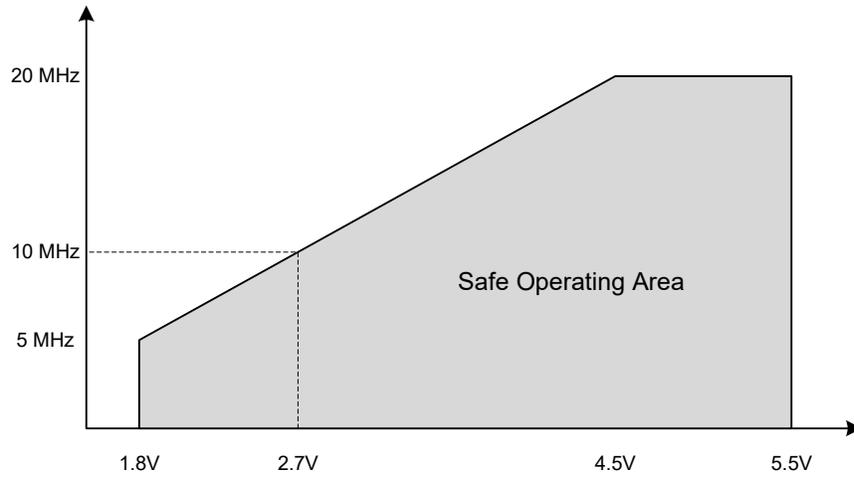
Figure 32-2. Maximum Frequency vs.  $V_{DD}$  for [105, 125]°C
