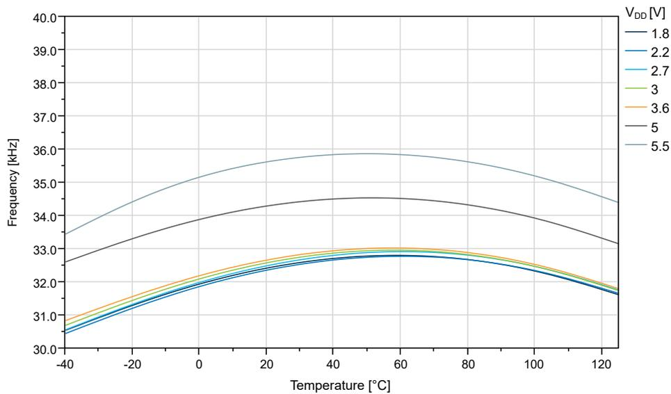
Figure 33-74. OSCULP32K Internal Oscillator: Frequency vs. V<sub>DD</sub>
