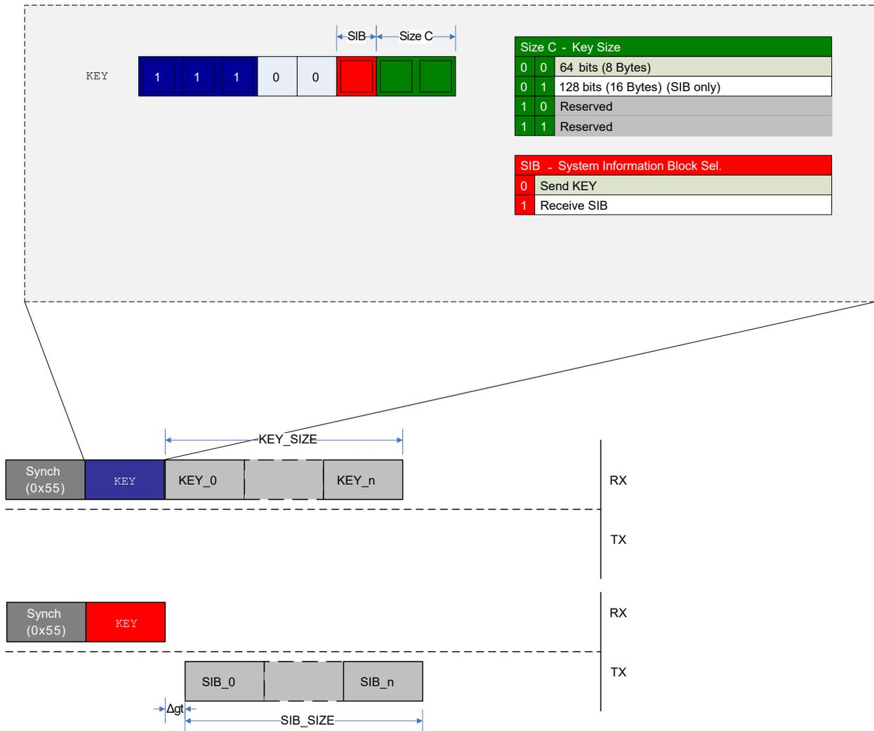
Figure 30-15 shows the transmission of a key and the reception of a SIB. In both cases, the Size C (`SIZE_C`) field in the operand determines the number of frames being sent or received. There is no response after sending a `KEY` to the UPDI. When requesting the SIB, data will be transmitted from the UPDI according to the current guard time setting.
