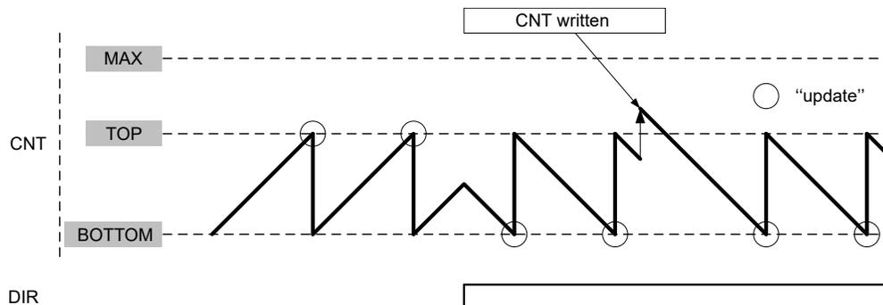
It is possible to change the counter value in the Counter (TCAn.CNT) register when the counter is running. The write access to TCAn.CNT register has higher priority than count, clear or reload, and will be immediate. The direction of the counter can also be changed during normal operation by writing to the Direction (DIR) bit in the Control E (TCAn.CTRLE) register.
