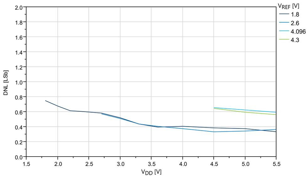
**Figure 33-57. DNL vs.  $V_{REF}$  ( $V_{DD} = 5.0V$ ,  $f_{ADC} = 115$  ksp/s, REFSEL = External Reference)**
