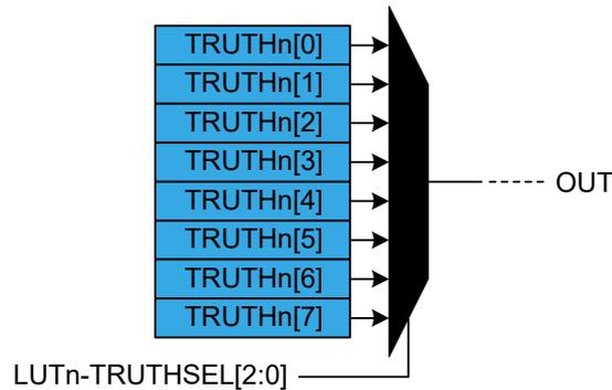
The truth table inputs (LUTn-TRUTHSEL[2:0]) are configured by writing the Input Source Selection bit fields in the LUT Control registers:
