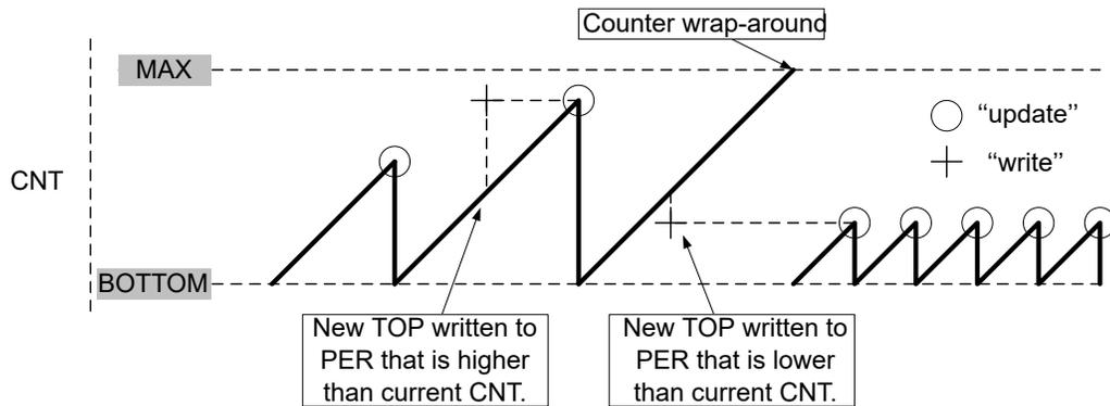
A counter wrap-around can occur in any mode of operation when counting up without buffering, as the TCA<sub>n</sub>.CNT and TCA<sub>n</sub>.PER registers are continuously compared. If a new TOP value is written to TCA<sub>n</sub>.PER that is lower than the current TCA<sub>n</sub>.CNT, the counter will wrap first, before a compare match occurs.
