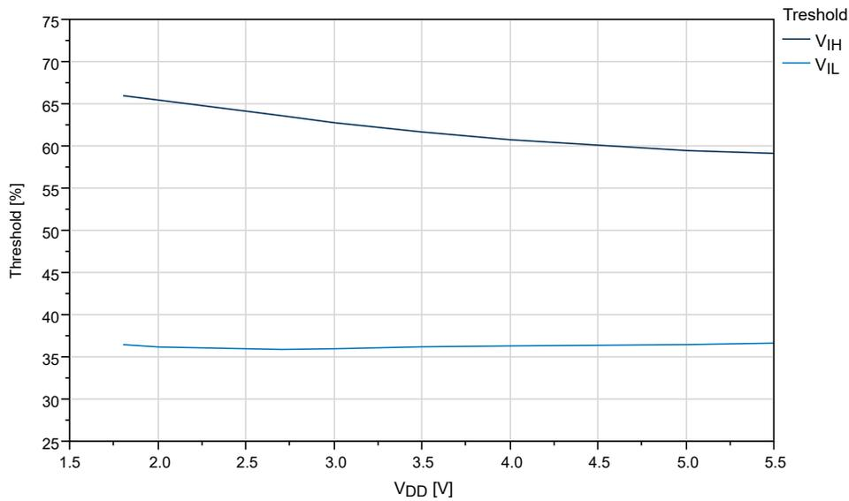
**Figure 33-21. I/O Pin Input Threshold Voltage vs.  $V_{DD}$  ( $V_{IH}$ )**
