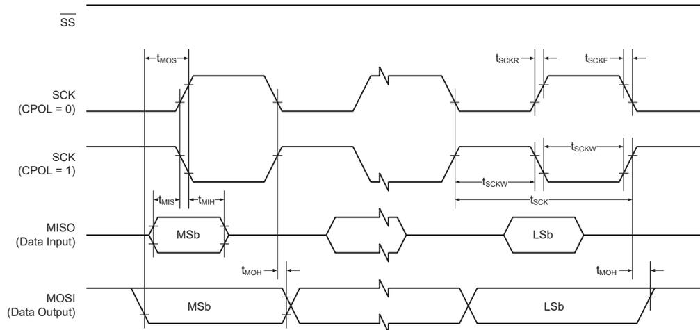
**Table 32-18. USART in SPI Host Mode - Timing Characteristics<sup>(1)</sup>**
