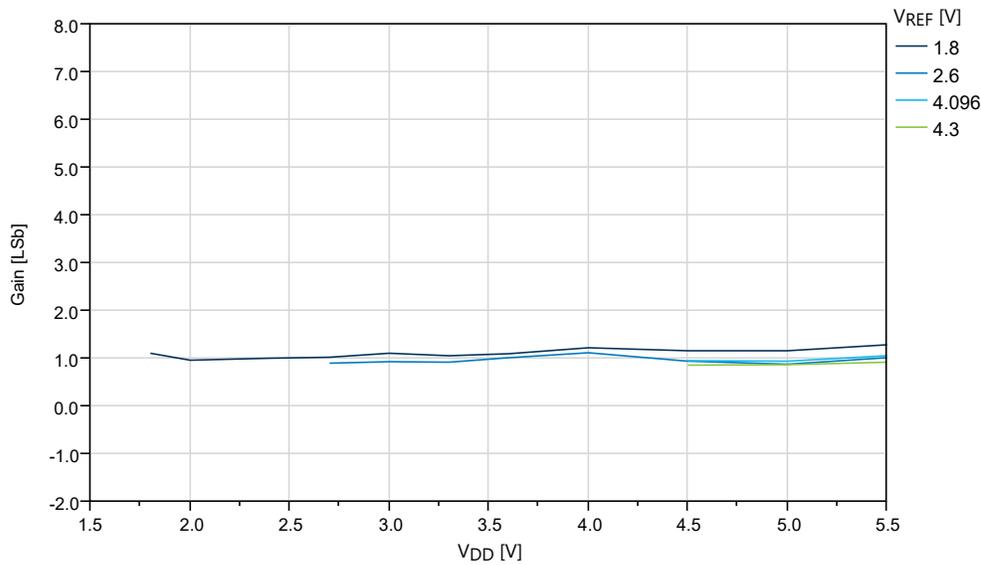
**Figure 33-59. Gain vs.  $V_{REF}$  ( $V_{DD} = 5.0V$ ,  $f_{ADC} = 115$  ksps, REFSEL = External Reference)**
