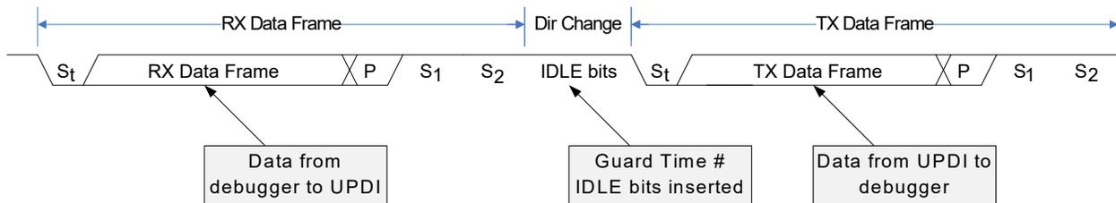
The UPDI guard time is the minimum Idle time that the connected debugger will experience when waiting for data from the UPDI. The maximum Idle time is the same as time-out. The Idle time before a transmission will be more than the expected guard time when the synchronization time plus the data bus accessing time is longer than the guard time.
