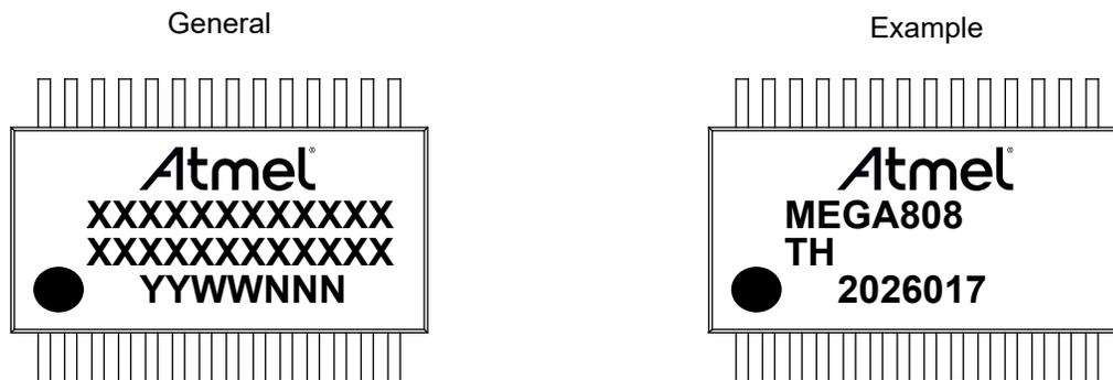
Figure 35-3. 32-Pin TQFP
