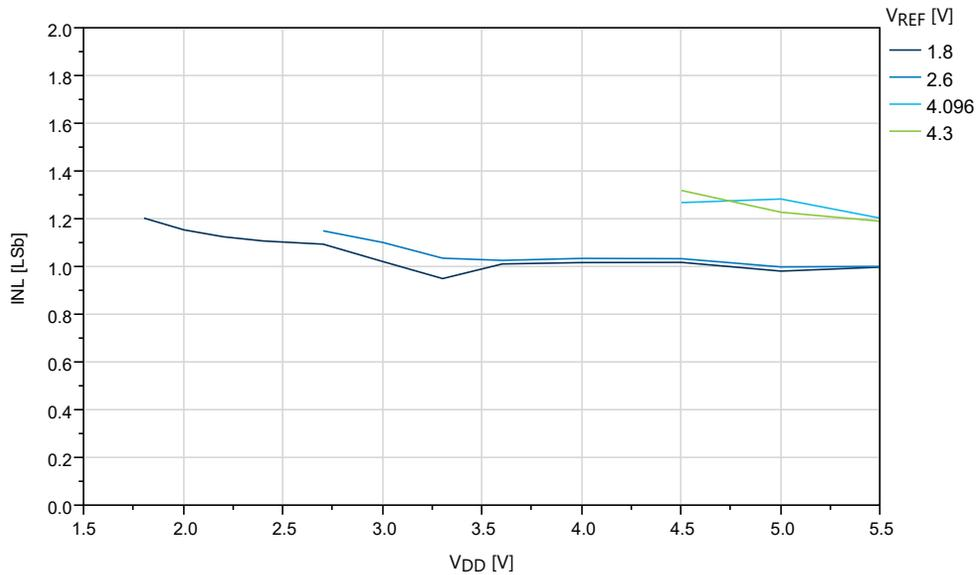
**Figure 33-61. INL vs.  $V_{REF}$  ( $V_{DD} = 5.0V$ ,  $f_{ADC} = 115$  kps, REFSEL = External Reference)**
