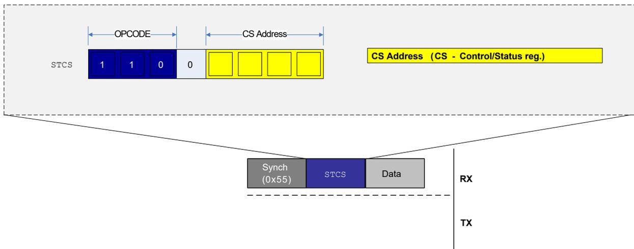
Figure 30-12 shows the data frame transmitted after the SYNCH character and the instruction frames. The STCS instruction byte can be immediately followed by the data byte. There is no response generated from the STCS instruction, as is the case for the ST and STS instructions.
