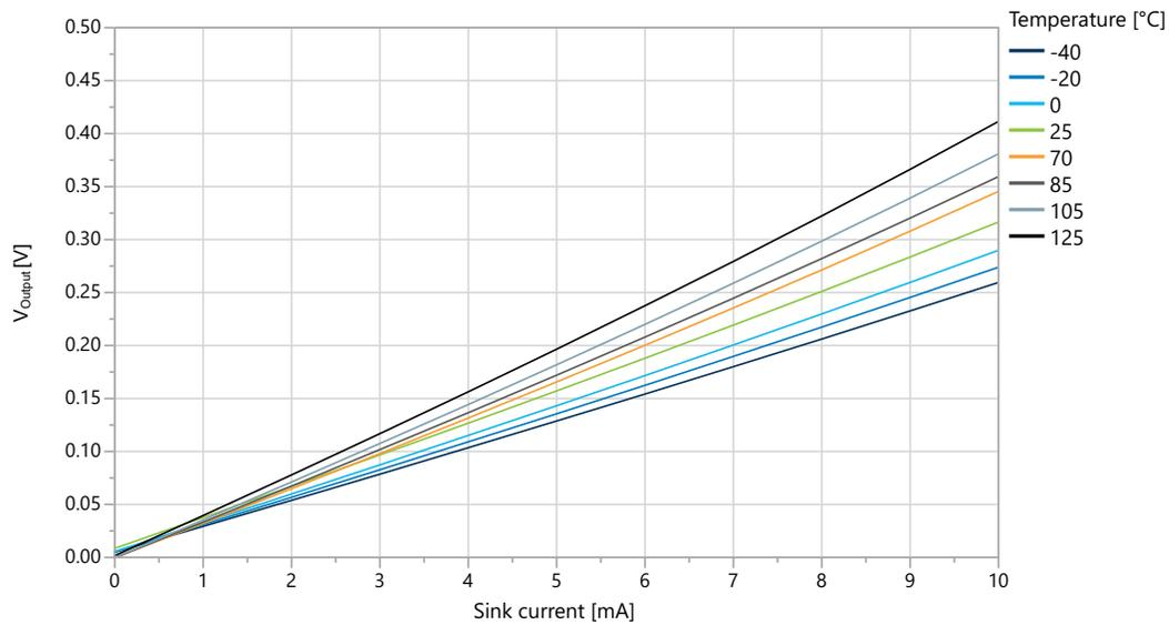
**Figure 33-25. I/O Pin Output Voltage vs. Sink Current ( $V_{DD} = 5.0V$ )**
