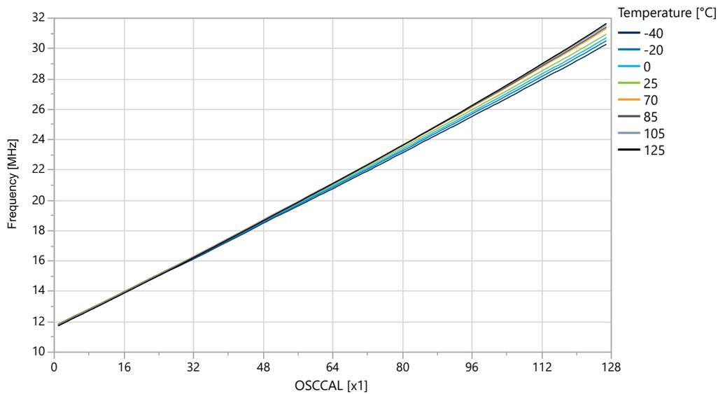
**Figure 33-71. OSC20M Internal Oscillator: Frequency vs. Temperature**
