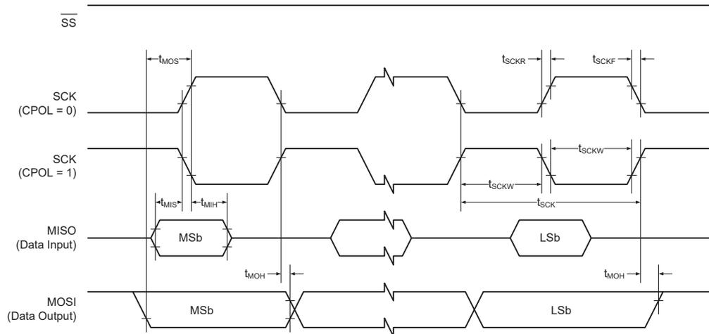
**Figure 32-8. SPI - Timing Requirements in Client Mode**
