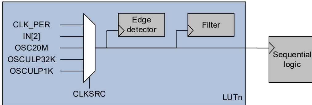
When the Clock Source (CLKSRC) bit is written to  $0x1$ , LUTn-TRUTHSEL[2] is used to clock the corresponding filter and edge detector (CLK\_LUTn). The sequencer is clocked by the CLK\_LUTn of the even LUT in the pair. When CLKSRC is written to  $0x1$ , LUTn-TRUTHSEL[2] is treated as OFF (low) in the TRUTH table.
