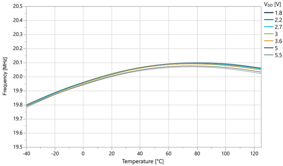
**Figure 33-72. OSC20M Internal Oscillator: Frequency vs. V<sub>DD</sub>**
