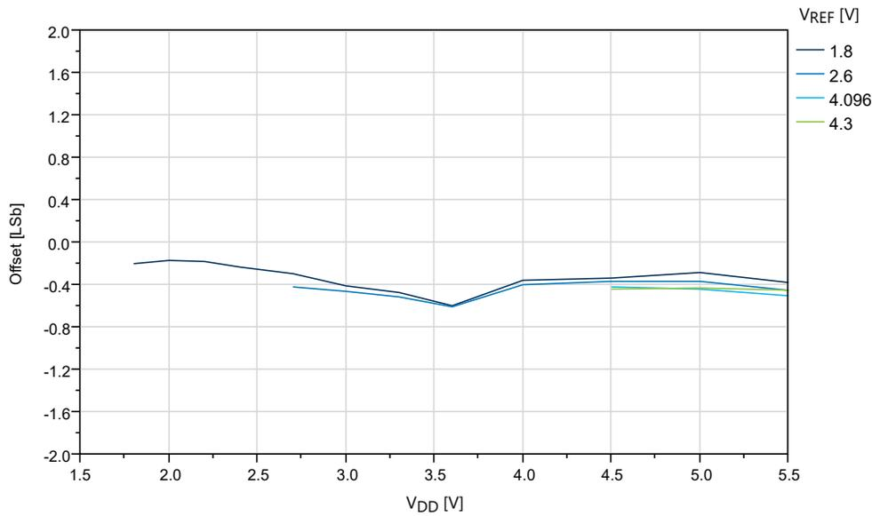
**Figure 33-63. Offset vs.  $V_{REF}$  ( $V_{DD} = 5.0V$ ,  $f_{ADC} = 115$  ksp/s, REFSEL = External Reference)**
