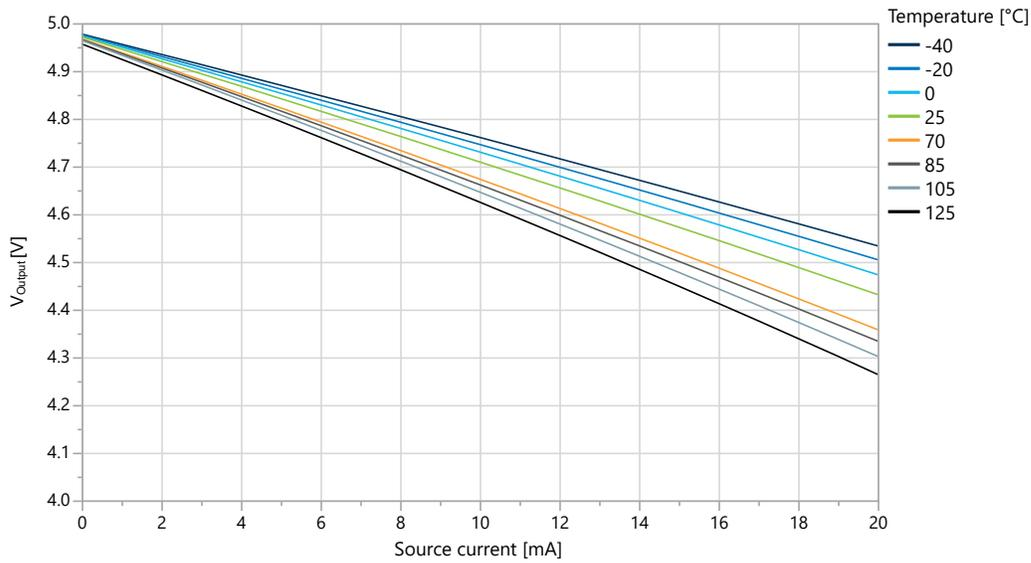
**Figure 33-30. I/O Pin Output Voltage vs. Source Current ( $T = 25^{\circ}C$ )**
