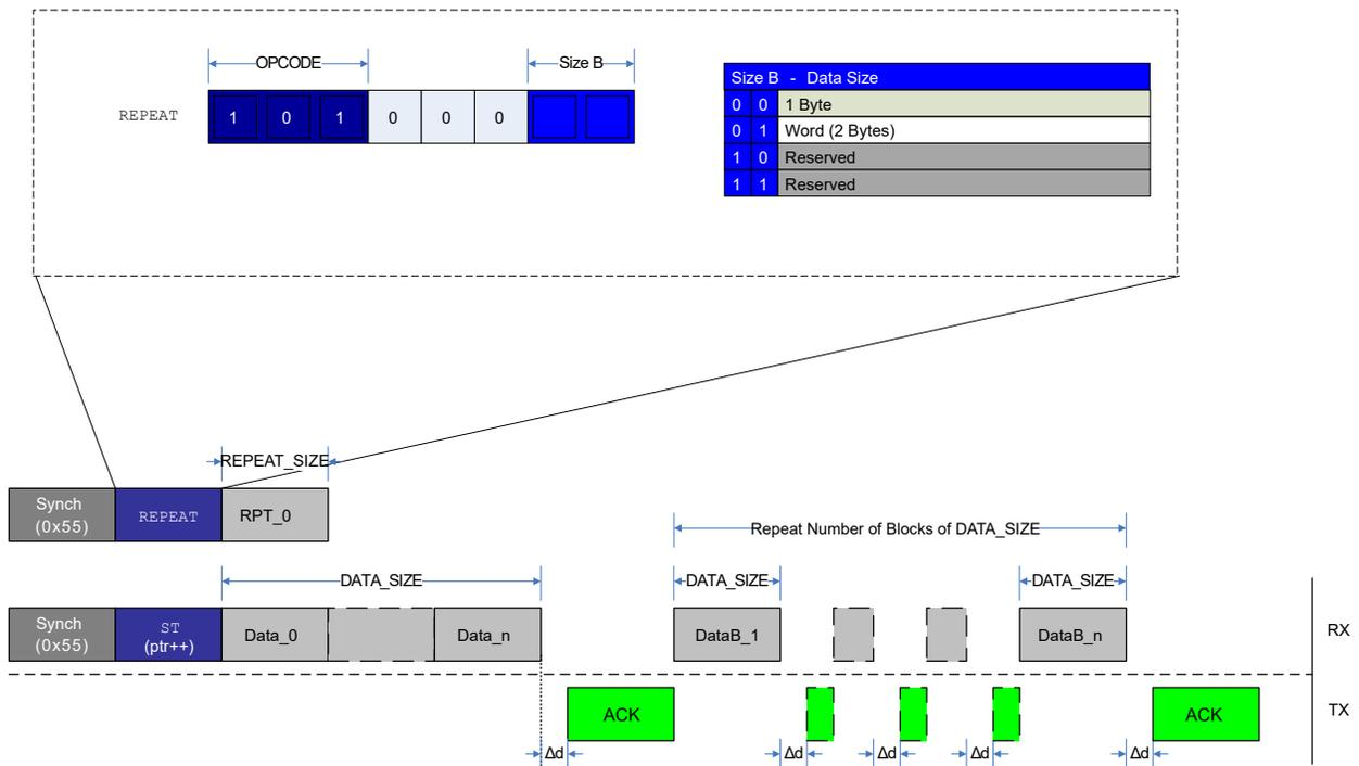
Figure 30-13 gives an example of a repeat operation with an ST instruction using pointer post-increment operation. After the REPEAT instruction is sent with  $RPT\_0 = n$ , the first ST instruction is issued with SYNCH and instruction frame, while the next  $n$  ST instructions are executed by only sending data bytes according to the ST operand DATA\_SIZE, and maintaining the Acknowledge (ACK) handshake protocol.
