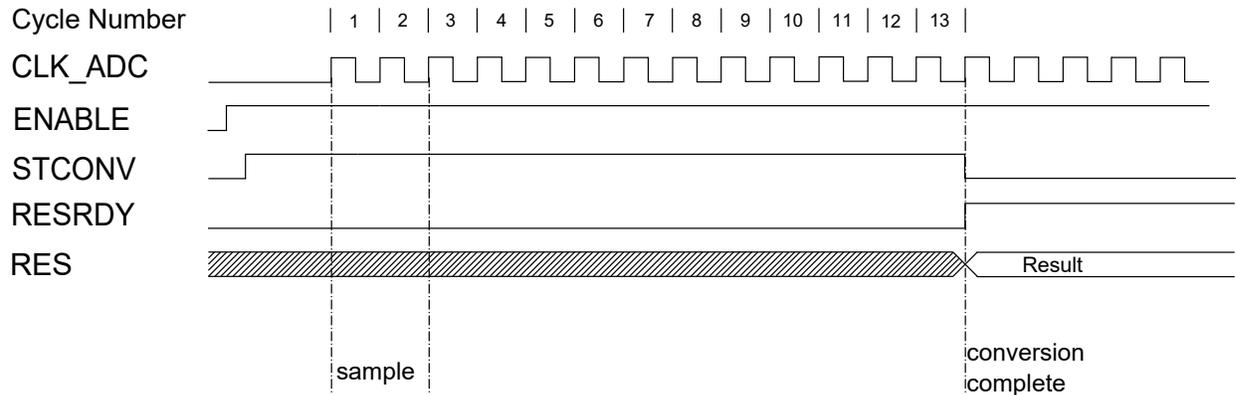
Both sampling time and sampling length can be adjusted using the Sample Delay bit field in the Control D (ADCn.CTRLD) register and the Sample Length bit field in the Sample Control (ADCn.SAMPCTRL) register. Both of these control the ADC sampling time in some CLK\_ADC cycles. This allows sampling of high-impedance sources without relaxing conversion speed. See the register description for further information. Total sampling time is given by:
