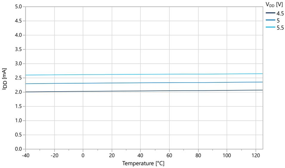
**Figure 33-12. Idle Supply Current vs. V<sub>DD</sub> (f = 32.768 kHz OSCULP32K)**
