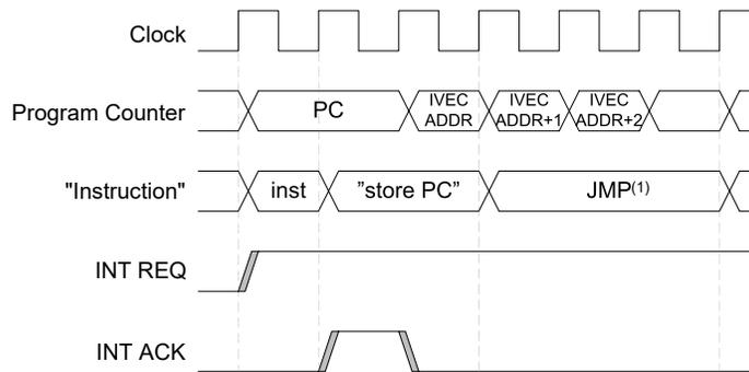
If an interrupt occurs during the execution of a multi-cycle instruction, the instruction is completed before the interrupt is served, as shown in the following figure.
