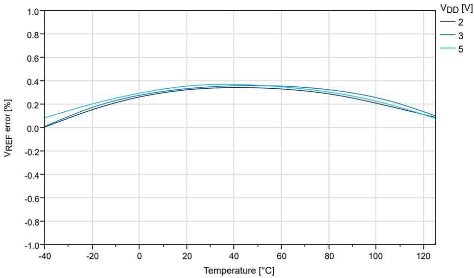
**Figure 33-35. Internal 1.1V Reference vs. Temperature**
