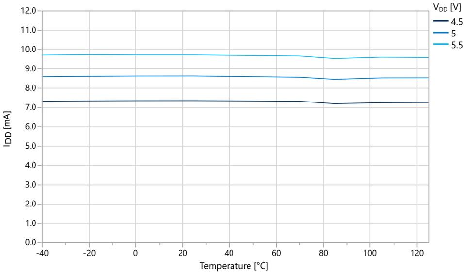
**Figure 33-4. Active Supply Current vs. Temperature (f = 16 MHz)**
