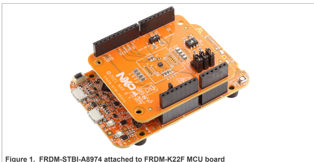
Figure 1. FRDM-STBI-A8974 attached to FRDM-K22F MCU board
