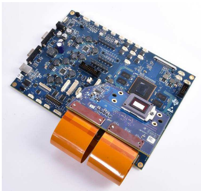
Figure 1. DLP DLPDLCR660TEVM and DLPLCRDC4422EVM Evaluation Module
