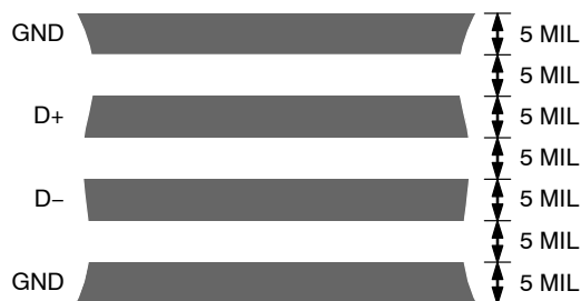
Figure 22. Typical Arrangement of Signal Tracks
