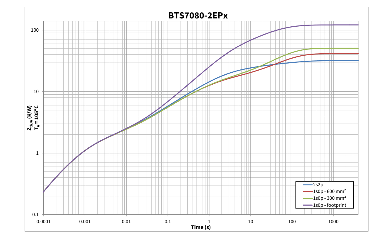
Figure 9 Typical Thermal Impedance. PCB setup according Chapter 4.4.1
