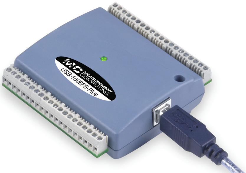
The USB-1608FS-Plus features simultaneous sampling of 8 analog inputs, and also provides 8 DIO lines and a 32-bit event counter
