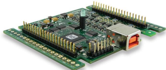
*The USB-1608FS-Plus-OEM has the same specifications as the USB-1608FS-Plus, but comes in a board-only form factor with header connectors instead of screw terminals.*
