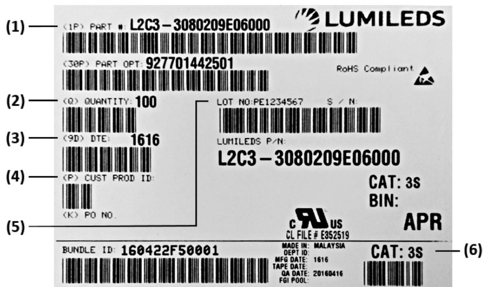
Figure 10. Example of inner box label for LUXEON SunPlus CoB Line.
