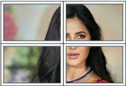
Correct Bezel Compensation
