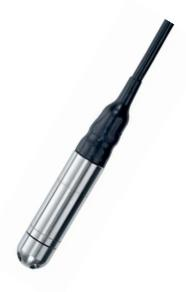
The ILSU is designed for use in continuous submersion in liquids such as water, oil and other non-aggressive chemicals. The submersible uses the latest piezo-resistive media-isolated silicon sensing technology and a stainless steel diaphragm within a 316L stainless steel housing.
