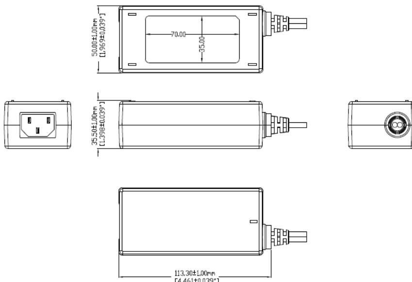
Alternative housing with waterproof barrier. Product PN# ends with suffix "RG"
