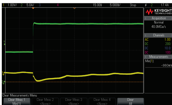
Inrush Current; 264Vac Input, Cold Start, Full Load; 31.4Apk
