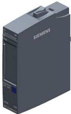
SIMATIC ET 200SP, Analog input module, AI 2x U/I 2-/4-wire High Feat., suitable for BU type A0, A1, Color code CC05, channel diagnostics, 16 bit, +/-0.1%
