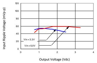
Figure 27. Input ripple voltage for various output with 2x150  $\mu$ F polymer and 2x47  $\mu$ F ceramic capacitors at the input (80% of lo,max).
