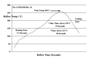
Figure 37. Recommended linear reflow profile using Sn/Ag/Cu solder.
