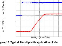
Figure 16. Typical Start-Up with application of Vin (Vin = 5.0Vdc, Vo = 3.3Vdc, Io = 6A).
