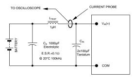
NOTE: Measure input reflected ripple current with a simulated source inductance ( $L_{TST}$ ) of 1µH. Capacitor C<sub>S</sub> offsets possible battery impedance. Measure current as shown above.
