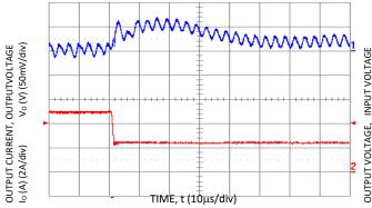
Figure 13. Transient Response to Dynamic Load Change from 100% of 50% full load (Vo = 3.3Vdc, Cext =  $2x150 \mu F$  Polymer Capacitors).
