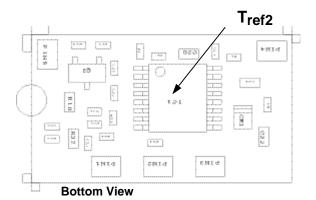
Figure 32. Tref Temperature measurement location.
