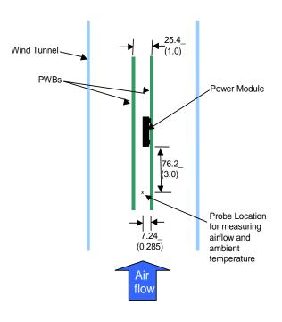
Figure 33. Thermal Test Set-up.
