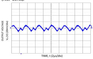
Figure 8. Typical Output Ripple and Noise (Vin = 5.0V dc, Vo = 0.75 Vdc, Io=6A).
