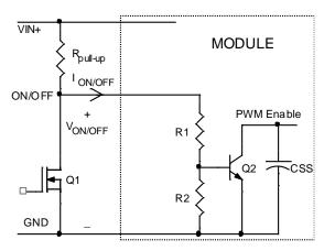
Figure 29. Circuit configuration for using negative logic On/OFF.
