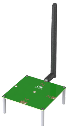
On edge of ground plane, bent 90 degrees
