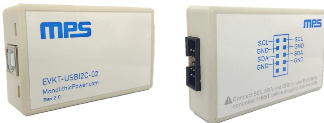
Figure 3: EVKT-USBI2C-02 Communication Interface
