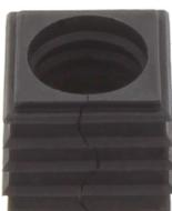
Seal, Mounting type: Plug in, Length x width: 20.3 mm, Max. cable diameter: 15 mm, IP 66, Colour: Black
