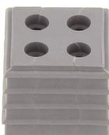
Seal, Mounting type: Plug in, Length x width: 20.3 mm, Max. cable diameter: 5 mm, IP 66, Colour: Grey
