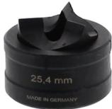
Sheet metal punch for round cutouts, Cutout diameter: 25.4 mm, Maximum wall thickness: 2.0 mm for S 235 sheet metal, Material: steel
