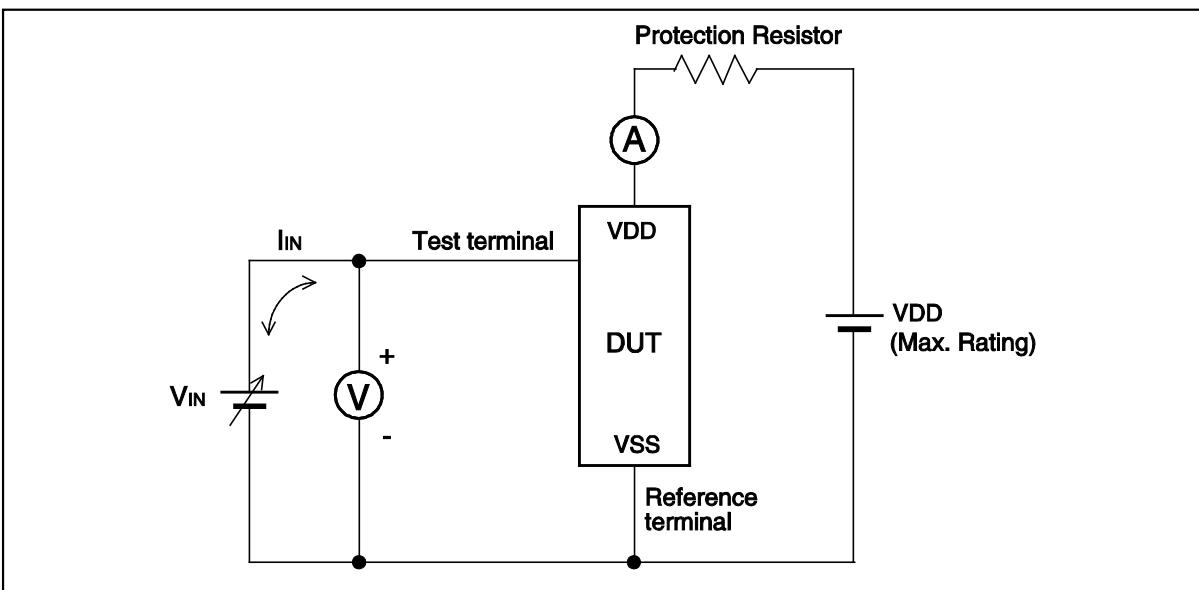
Note: The voltage  $V_{\text{IN}}$  is increased gradually and the current  $I_{\text{IN}}$  of 300 mA at maximum shall flow.
