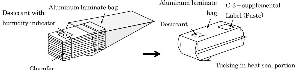
**(4) Put the aluminum laminate in inner-holder, store in inner box.**
