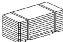
**(3) Put desiccant(with humidity indicator:20g) on the bundled trays, vacuum pack in aluminum laminate bag, then seal and paste label for inner box.**
