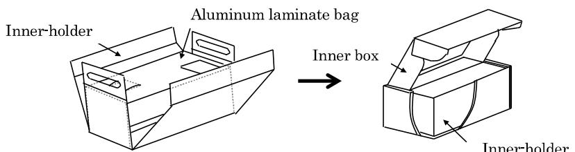
**(5) Close the lids of the inner box, paste one label for inner box.**
