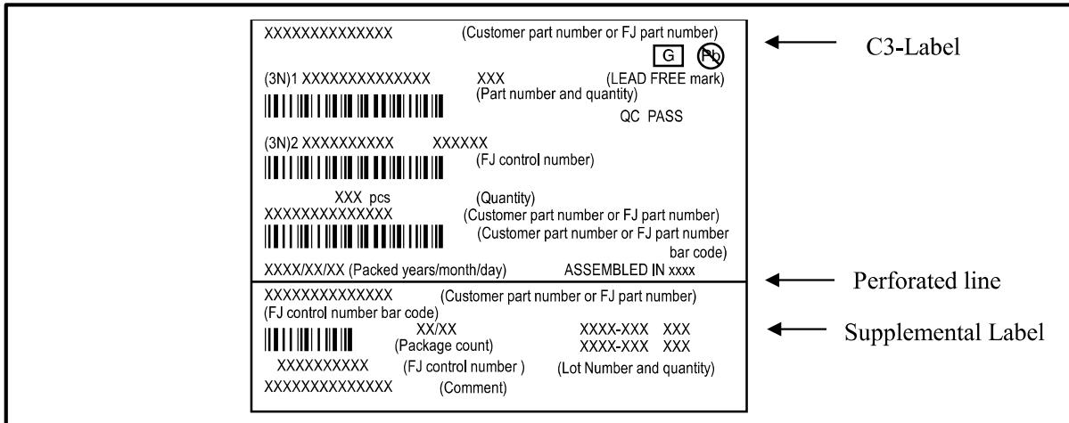
Label II-A: Label on Outer box [D Label] (100mm x 100mm)
