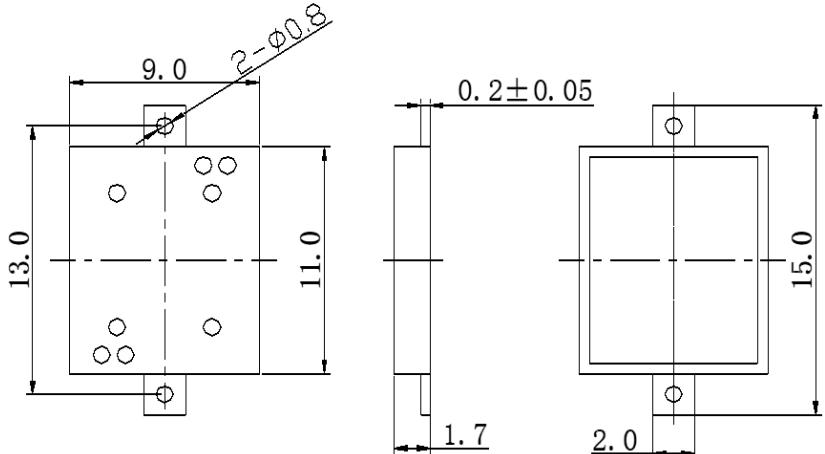
Tolerance:  $\pm 0.5$  (unit:mm), unless otherwise specified.
