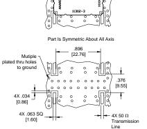
Dimensions are in Inches [Millimeters] 11302-3 Mounting Footprint
