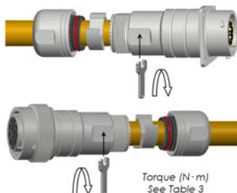
Step 10: Assemble back shell
