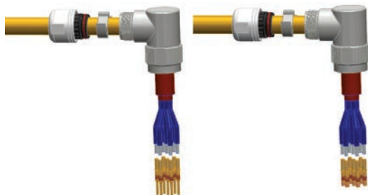
Step 7: Attach contacts to wire leads
