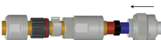
Step 6: Slide plug onto crimped terminal assembly
