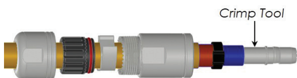
Step 5: Crimp terminal to conductor
