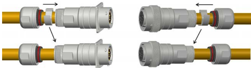
Step 11: Push shielding clip into backshell
