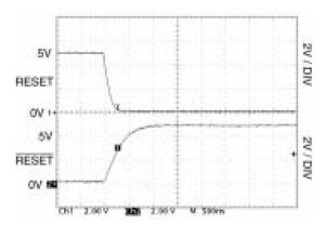
Fig. 13: SP707 RESET and RESET De-Assertion
