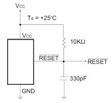
Fig. 11: SP705/707 RESET Response Time Circuit
