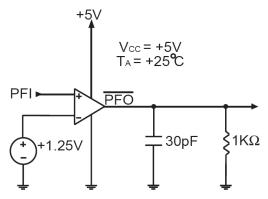
Fig. 5: Power-Fail Comparator De-Assertion Response Time Circuit
