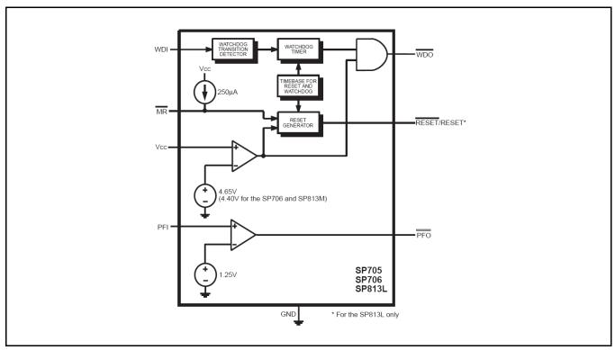
Fig. 1: SP705-SP706-SP813L Block Diagram
