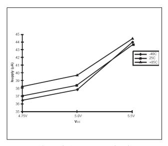
Fig. 25: Supply Current vs. Supply Voltage
