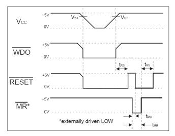
Fig. 19: SP705/706 Timing Diagrams with WDI tri-stated.
