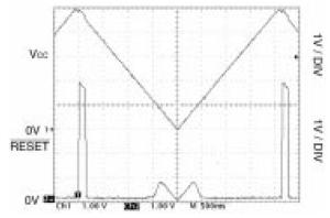
Fig. 8: SP705/707 RESET Output Voltage vs. Supply Voltage
