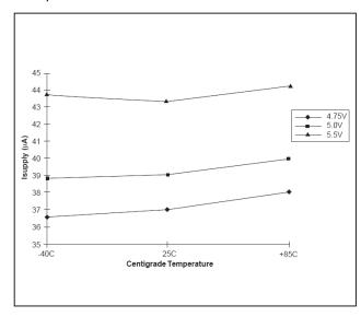
Fig. 24: Supply Current vs. Temperature
