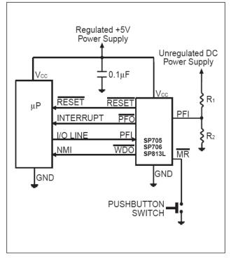
Fig. 20: Typical Operating Circuit
