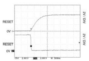
Fig. 12: SP707 RESET and RESET Assertion
