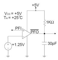
Fig. 7: Power-Fail Comparator Assertion Response Time Circuit
