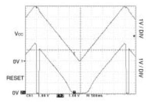
Fig. 15: SP707/708/813L RESET Output Voltage vs. Supply Voltage
