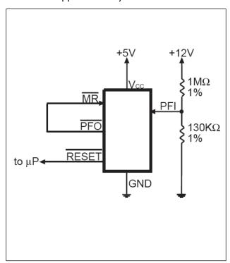
Fig. 21: Monitoring +5V and +12V Power Supplies
