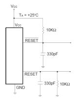
Fig. 14: SP707 RESET and RESET Assertion and De-Assertion Circuit
