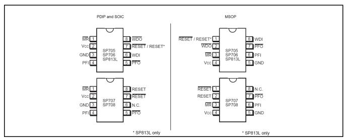
Fig. 3: Pin Assignment
