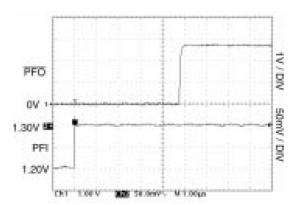
Fig. 4: Power-Fail Comparator De-Assertion Response Time
