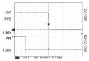
Fig. 6: Power-Fail Comparator Assertion Response Time
