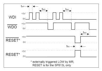
Fig. 18: SP705/706/813L Watchdog Timing Waveforms
