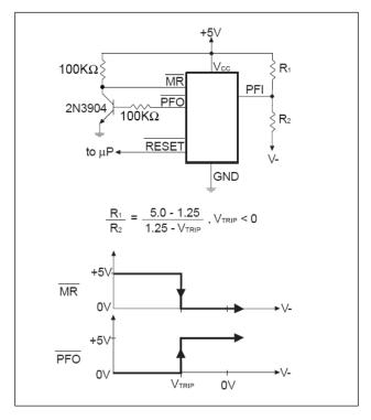
Fig. 22: Monitoring a Negative Voltage Supply
