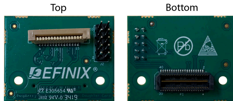
Figure 1: Raspberry Pi Camera Connector Daughter Card
