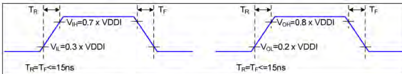
Figure 2 Rising and Falling Timing for I/O Signal
