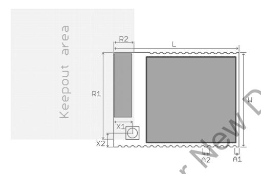
Figure 7. ETRX3 Physical Dimensions
