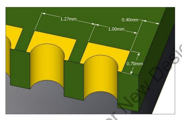
Figure 8. Typical pad dimensions
