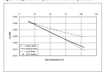
Figure 10: 2000K, 65 CRI Color Shift vs. Case Temperature
