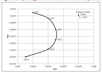
Figure 13: 3000K, 90 CRI Color Shift vs. Case Temperature<sup>1,3</sup>
