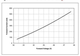
Figure 3: Vero SE 10D Drive Current vs. Voltage
