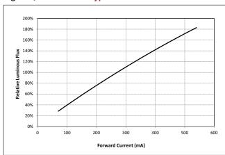
Figure 6 Vero 10D SE Typical Relative Flux vs. Current
