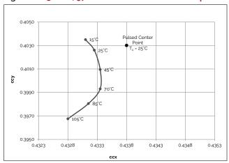
Figure 14: 3000K Class A Color Shift vs. Case Temperature<sup>1</sup>
