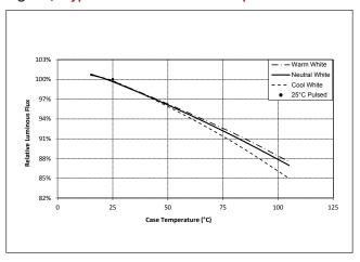
Figure 9: Typical DC ccx Shift vs. Case Temperature
