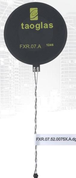
The FXR.07.52.0075X.A.dg is an NFC Ferrite antenna on 75mm twisted pair 28AWG cable with ACH(F) connector. It works with specific NFC chips which need to connect via JST ACH connector.
