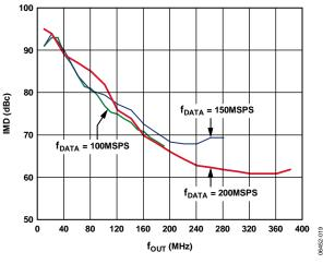
Figure 20. AD9779A Third-Order IMD vs. f<sub>OUT</sub>, 4× Interpolation
