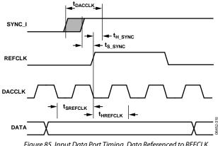
Figure 85. Input Data Port Timing, Data Referenced to REFCLK,  $f_{DACCLK} = f_{REFCLK} \times 4$
