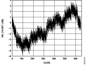
Figure 6. AD9779A Typical INL
