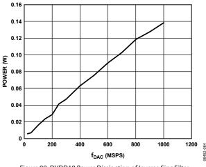
Figure 99. DVDD18 Power Dissipation of Inverse Sinc Filter
