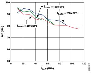
Figure 18. AD9779A Third-Order IMD vs. four, 1× Interpolation
