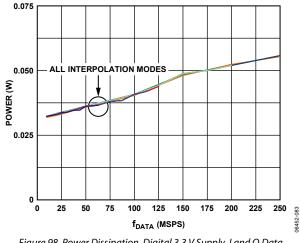
Figure 98. Power Dissipation, Digital 3.3 V Supply, I and Q Data, Dual DAC Mode
