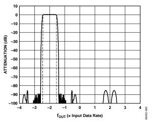
Figure 63. Interpolation/Modulation Combination of –2f<sub>DAC</sub>/8 Filter
