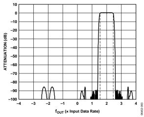
Figure 66. Interpolation/Modulation Combination of 2fDAC/8 Filter
