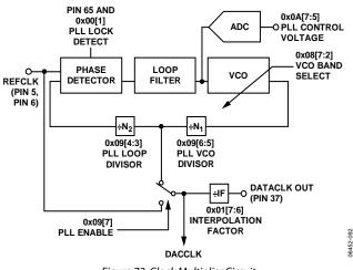
Figure 72. Clock Multiplier Circuit
