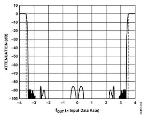
Figure 61. Interpolation/Modulation Combination of 4f<sub>DAC</sub>/8 Filter
