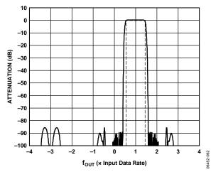
Figure 65. Interpolation/Modulation Combination of f<sub>DAC</sub>/8 Filter
