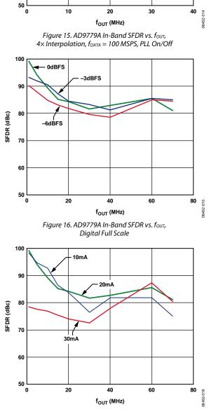
Figure 17. AD9779A In-Band SFDR vs. four, Output Full-Scale Current
