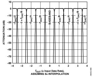
Figure 69. Nonshifted Bandwidths Accessible with the Filter Architecture
