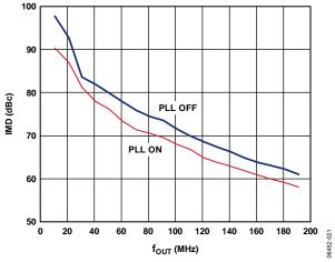
Figure 22. AD9779A Third-Order IMD vs. fout, 4× Interpolation, f<sub>DATA</sub> = 100 MSPS, PLL On/Off
