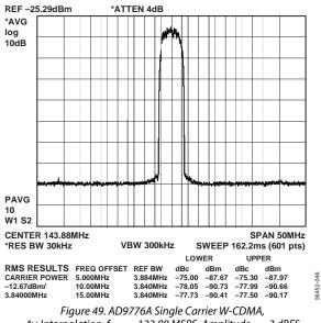
$4 \times$  Interpolation,  $f_{DATA} = 122.88$  MSPS, Amplitude = -3 dBFS
