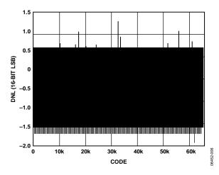
Figure 7. AD9779A Typical DNL
