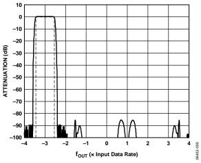
Figure 62. Interpolation/Modulation Combination of -3f<sub>DAC</sub>/8 Filter
