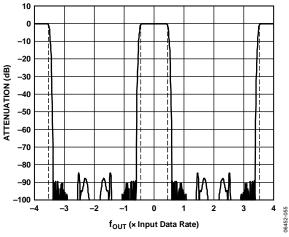
Figure 58. 4× Interpolation, Low-Pass Response to ±4× Input Data Rate (Dotted Lines Indicate 1 dB Roll-Off)
