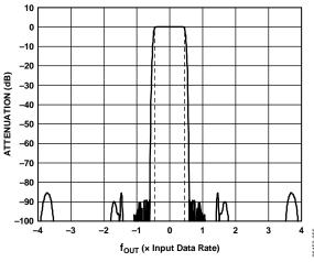
Figure 59. 8× Interpolation, Low-Pass Response to ±4× Input Data Rate (Dotted Lines Indicate 1 dB Roll-Off)
