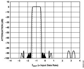
Figure 64. Interpolation/Modulation Combination of –f<sub>DAC</sub>/8 Filter
