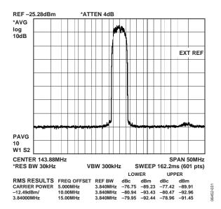
Figure 32. AD9779A W-CDMA Signal, 4× Interpolation, f<sub>DATA</sub> = 122.88 MSPS, f<sub>DAC</sub>/4 Modulation
