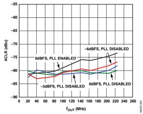
Figure 34. AD9779A ACLR for Third Adjacent Band W-CDMA, 4× Interpolation, f<sub>DATA</sub> = 122.88 MSPS, On-Chip Modulation Translates Baseband Signal to IF
