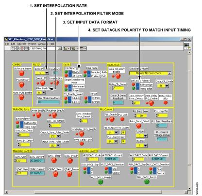
Figure 102. 3-Wire Interface Port Software Window
