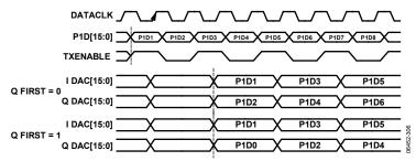
Figure 83. Single Port Mode Digital Interface Timing
