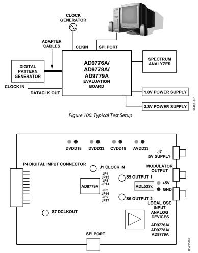
Figure 101. AD9776A/AD9778A/AD9779A Evaluation Board Showing All Connections
