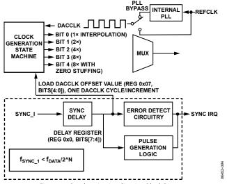
Figure 88. Synchronization Circuitry Block Diagram
