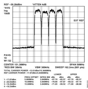
Figure 35. AD9779A Multicarrier W-CDMA Signal, 4× Interpolation, f<sub>DAC</sub> = 122.88 MSPS, f<sub>DAC</sub>/4 Modulation
