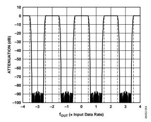
Figure 57. 2× Interpolation, Low-Pass Response to ±4× Input Data Rate (Dotted Lines Indicate 1 dB Roll-Off)
