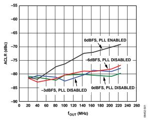
Figure 33. AD9779A ACLR for Second Adjacent Band W-CDMA, 4× Interpolation, f<sub>DATA</sub> = 122.88 MSPS, On-Chip Modulation Translates Baseband Signal to IF
