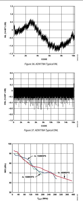
Figure 38. AD9778A IMD vs. fout, 4× Interpolation
