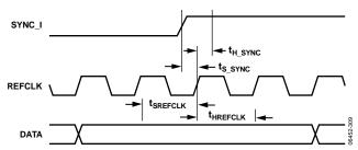
Figure 84. Input Data Port Timing, Data Referenced to REFCLK,  $f_{DACCLK} = f_{REFCLK}$
