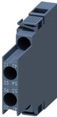
Auxiliary switch lateral, 1 NO + 1 NC Current path 1 NC, 1 NO for 3RH and 3RT screw terminal R: 21/22, 33/34 L: 41/42, 53/54
