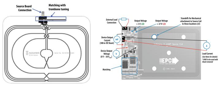
Figure 7: Proper connection for the source coil.
