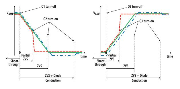
Figure 10: ZVS timing diagrams.
