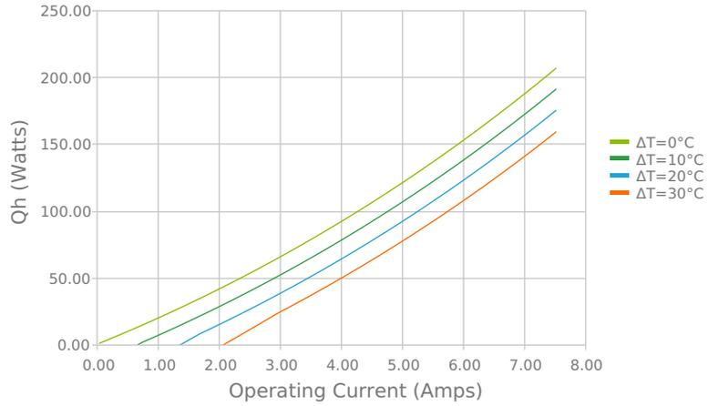
Total Heat Dissipated at Hot Side (Qh=Qc+Pin)
