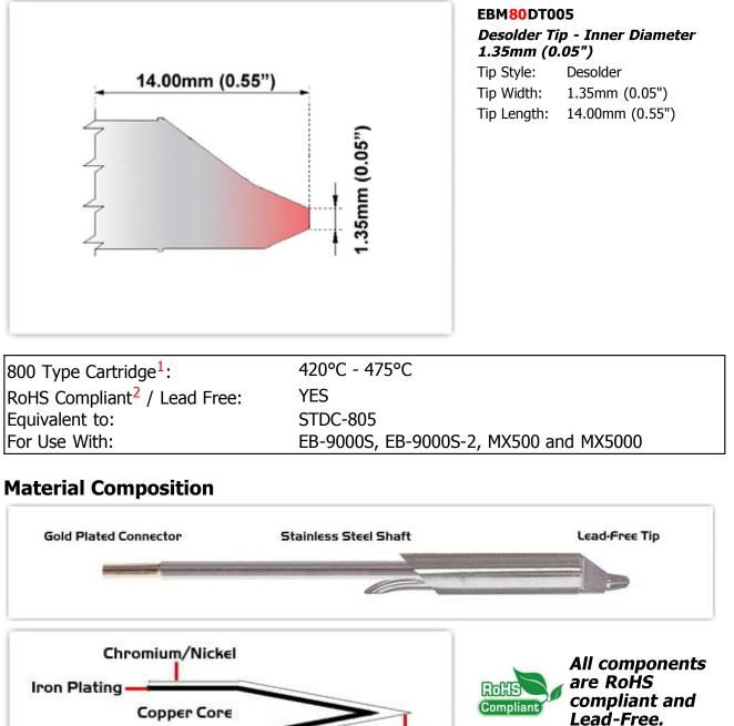
1 Easy Braid Co. tip cartridges will typically idle within a temperature range of +/-1.1°C. However, there is variation in idle temperature across tip geometries within an individual temperature series. Easy Braid Co. offers a wide variety of tip geometries from 0.25mm fine point tip to 5mm chisel. The length and geometry of a tip will have an influence on the tip idle temperature. To accurately measure idle temperature it will depend greatly on the measurement method,
