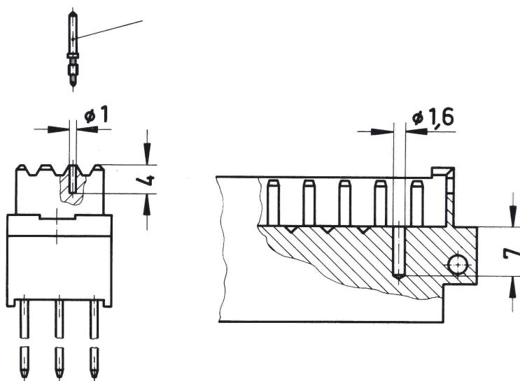
To avoid cross-plugging of adjacent connectors a coding system is required. With the aid of the marked indents between the contact rows of the male connector a hole has to be drilled at the desired position (also see drawing). The code pin can then be inserted into the corresponding cavity of the female connector by the means of the insertion tool.
