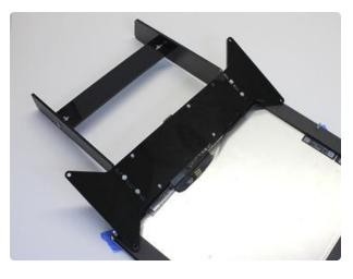
Now flip the bow tie / support over, remove the tape and tighten the four small screws.
