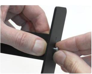
Slots in the leg pieces are "keyed" to fit into the tabs on the cross brace. Position a leg using these tabs and slots, then install a #4-40 1/2" screw through the middle, meeting up with the nut held in the cross brace.
