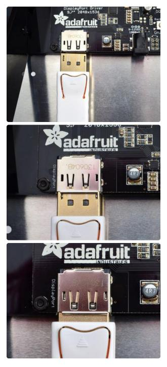
Removing a DisplayPort connector is a little more difficult because the connector is quite strong. You have to press down on the cable latch and wiggle-pull it out. Hold onto the connector with your other hand to make it easier!
