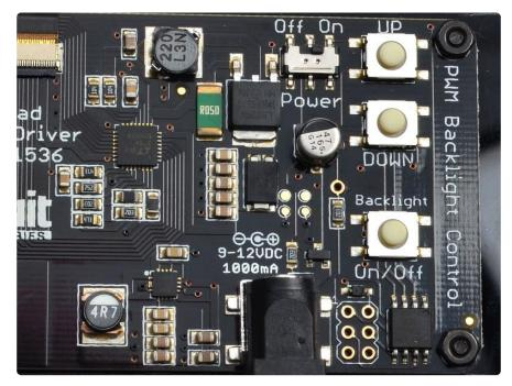
To control the backlight of the display, we use the awesome LT3754 LED driver from Linear Tech (https://adafru.it/d8V). The great thing about this driver is it is a cross between an efficient boost convert and a fully-matched constant-current LED driver. The boost converter half can take 9-12VDC and boost it up to ~22VDC and the LED driver half makes sure that each LED strand is driven with exactly 18.5mA for perfectly distributed light (which gives better color representation).
