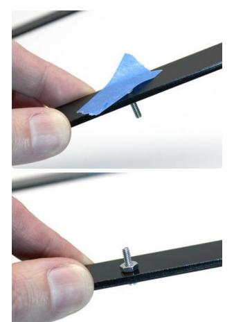
Insert a screw into each hole (1/2" or 5/8", as appropriate to the above diagram). The bezel will need to be flipped over later, so as you place each screw, secure it with a bit of tape, <u>or</u> you can use the nuts temporarily to keep the screws from sliding out (you'll need to remove these nuts later).
