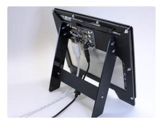
Stand the screen up and remove the tape pieces (if used) from the front bezel. Give it a <u>very gentle</u> tap on the desk to make sure everything's seated, then work around the perimeter tightening these screws. Just snug them down a little... don't go crazy or you'll crack the plastic.
