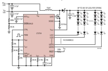
92% Efficient, 36W Backlight LED Driver
