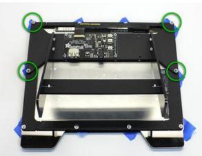
Carefully turn the stand over and lower it onto the four 5/8" screws. Add a nut to each and finger tighten.
