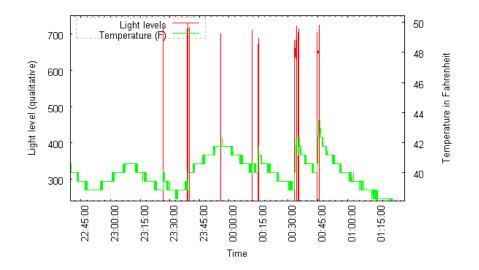
Zooming into the plot at about 12:40AM, we can see how the temperature climbs whenever the door is open, even in a few seconds it can climb 4 degrees very quickly!
