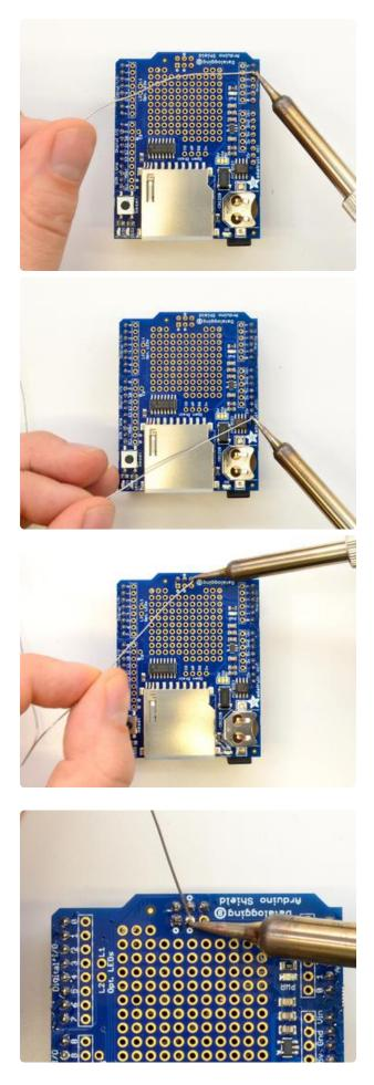
Flip around and solder the other side as well as the 2x3 header
