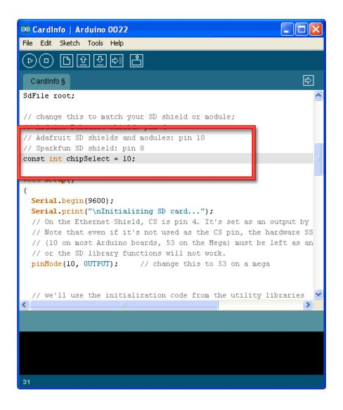
If you have the pre-rev B version of the Datalogger Shield, and you are using a Mega or Leonardo check here for now to adjust the pin setup (https://adafru.it/ref)
