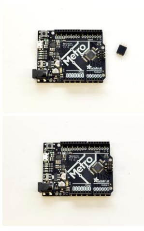
Place the 2x3 female header on to the Arduino/ Metro
