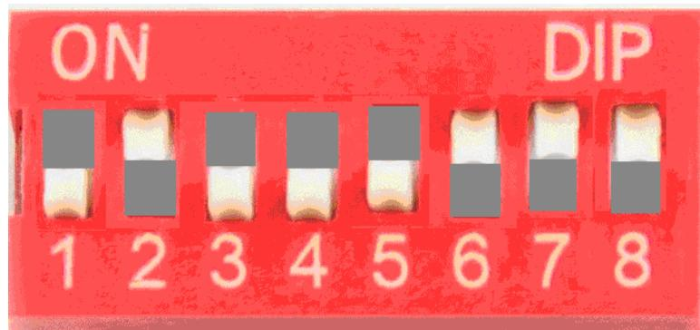
Set to this setting to enable operation for Motors with 0-10v controls
