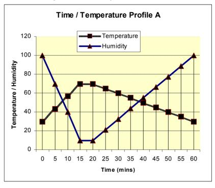
During the 6,000 hours life test, all test specimens must undergo the following:
