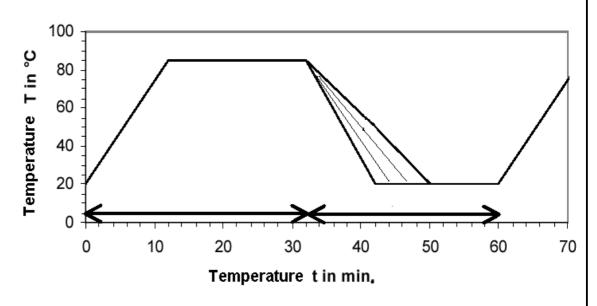
Prior to 4,000 hours life test, all test specimens must undergo the following:
