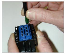
2. Once past the terminal opening, push the service tool against the terminal and push until it wedges between the terminal and the lock finger. Once the terminal lock finger is disengaged, gently pull on the wire to release the terminal. If the terminal resists, the service tool may not be fully engaged. Give the service tool a further push to ensure that it has disengaged the terminal lock finger.
