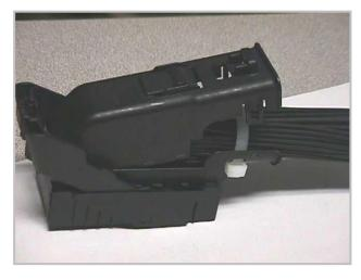
3. At this time the tie wrap should be removed from the wire bundle for easier access to the wire to be serviced.
