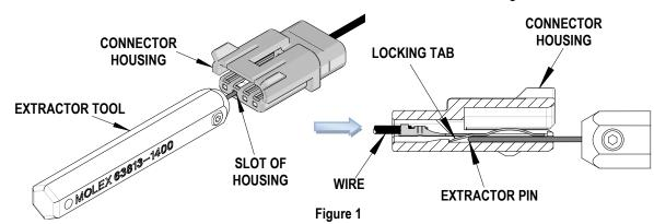
3. The extractor pin will depress the terminal locking tabs then pull the terminated wire out of the housing. Wiggling the wire while pulling it out will help.
