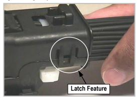
2. With wire dress cover latch features unlatched; insert finger into wire dress cover and pull up and away from the wire bundle.
